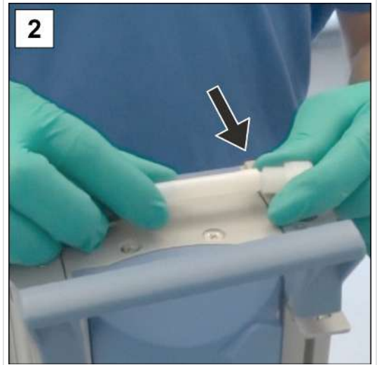
2. Rotate the angled screw fitting back into the molded hose by a quarter turn.
