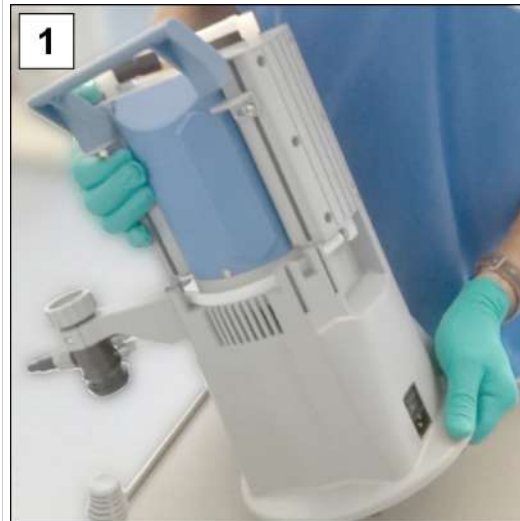
1. Set the pumping unit up-right.
