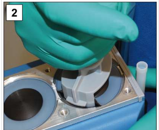
2. Carefully position the diaphragm wrench on the diaphragm support disc.
