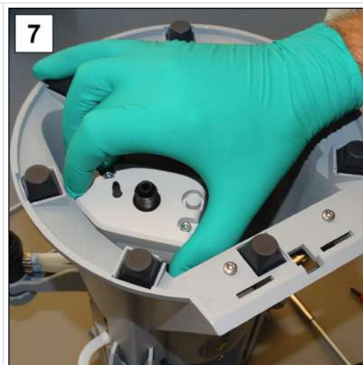
7. Disconnect the VACUUBUS connector at the bottom and remove the sensor.
