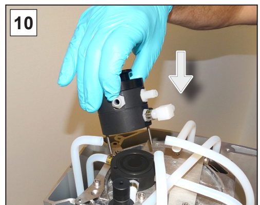
10. Position the suction distributor with screws and wind in the screw fittings until hand-tight; Phillips screwdriver size 2.
