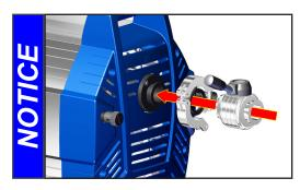
Use a suitable valve (see "Accessories / Spare parts", pg. 43) to isolate the pump from the vacuum application. This is to allow the pump to warm up before pumping condensable vapors and to clean the pump after use before it is switched off
