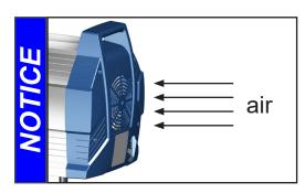
Make sure the fan's air supply is adequate. Do not place the pump on soft surfaces (e.g., rubber foam) during operation. This may reduce the air circulation in the pump housing and affect the fan's cooling effect. Check fan regularly for dust/dirt. Clean fan guard grill if necessary to avoid a reduction of ventilation.
