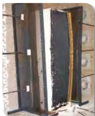
CHEMISAFE cabinet series FIRE MY11 AFTER fire resistance test.
