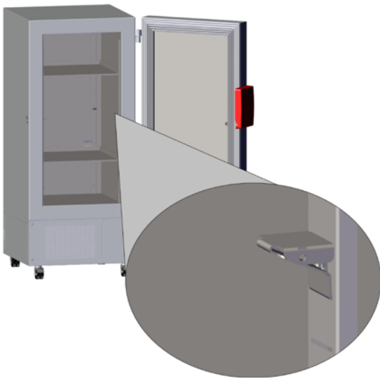
Figure 17: Inserting the shelf holders
